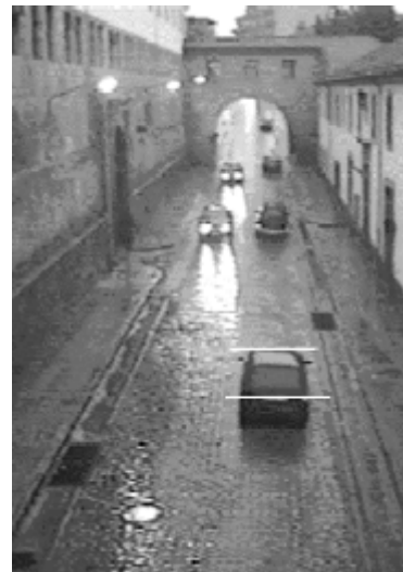
Figure 7. Situation where the vehicle's headlights cause some false detections.
