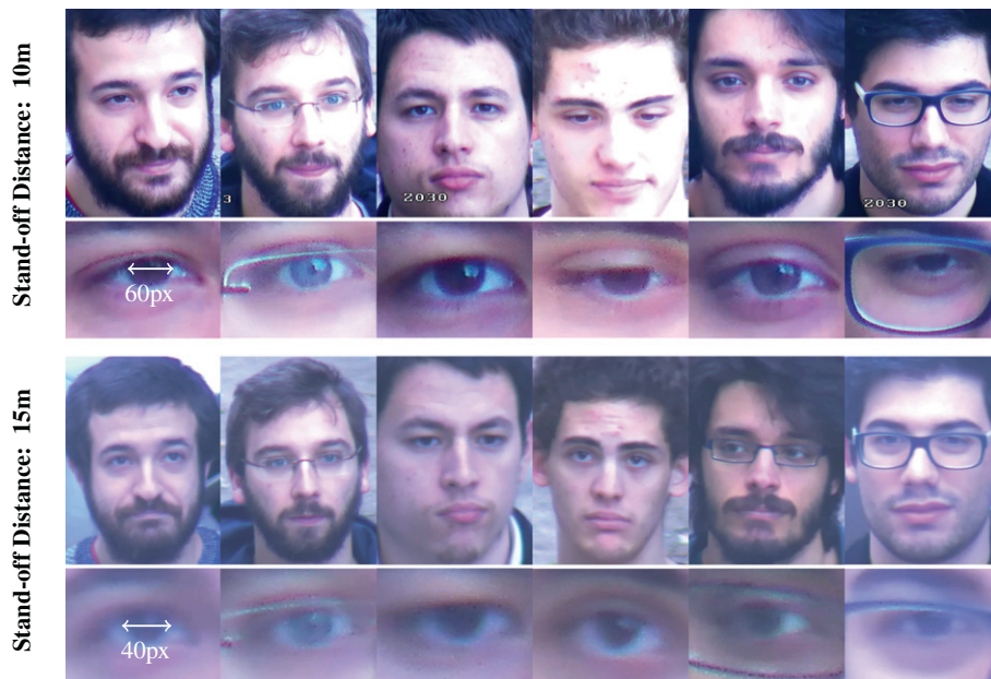
Fig. 3. Examples of facial data acquired in surveillance environments with the corresponding iris/periocular regions. The upper row contains samples acquired 10m away from the subjects, while the bottom row illustrates images acquired from 15m away.
