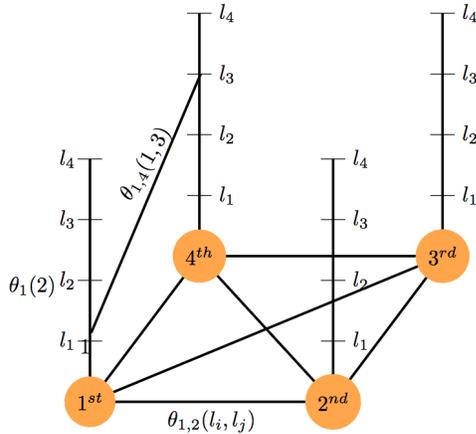
Fig. 4. Illustrative example (taken from [37]) of the MRF used when four targets are in the scene. Labels encode the set of targets in the scene, whereas the nodes correspond to the order that they will be imaged. Unary costs represent the angular differences between the current position of the camera and each target, whereas pairwise costs model the transition angles.
