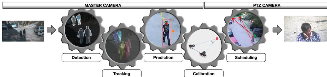
**Fig. 2. Processing chain of the QUIS-CAMPI surveillance system.** A master-slave architecture is adopted for the proposed surveillance system, where the master camera is responsible for monitoring a surveillance area and providing a set of interest regions (in this case the location of subjects face) to the PTZ camera.
