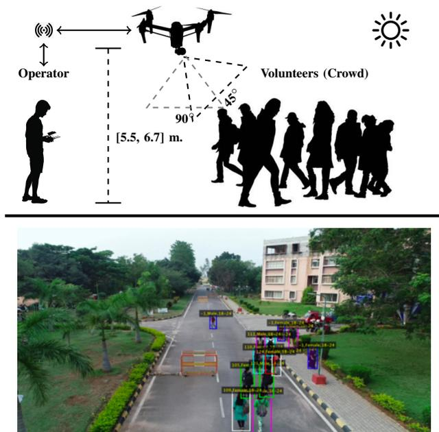
Fig. 2. At top: schema of the data acquisition protocol used. Human operators controlled DJI Phantom 4 aircrafts in various scenes of two university *campi*, flying at altitude between 5.5 and 6.7 meters, with gimbal pitch angles between  $45^\circ$  to  $90^\circ$ . The image at the bottom provides one example of a full scene of the P-DESTRE set.
