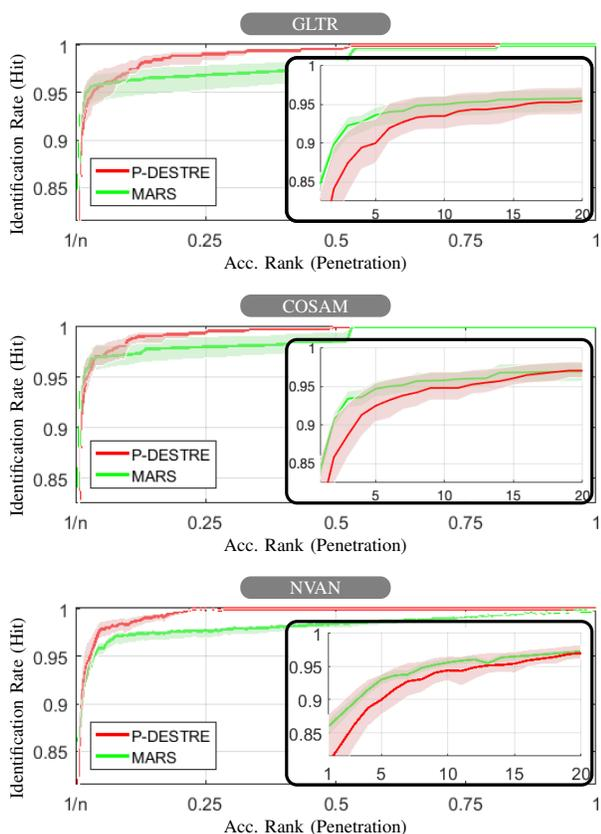
Fig. 8. Comparison between the closed-set identification (CMC) curves observed in the MARS (green lines) and P-DESTRE (red lines) sets for the GLTR, COSAM and NVAN re-identification techniques. Zoomed-in regions with the top-1 to 20 results are shown in the inner plots.
