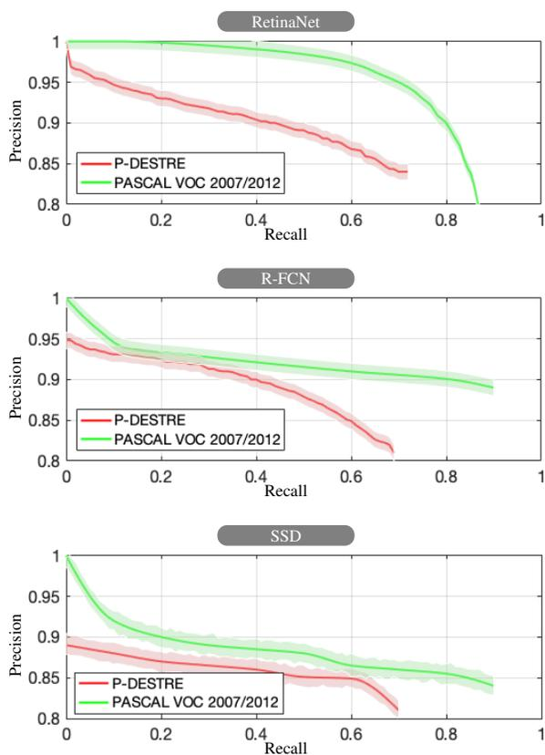
Fig. 5. Comparison between the precision/recall curves observed in the PASCAL VOC 2007/2012 (green lines) and P-DESTRE (red lines) sets. Results are given for the RetinaNet (top plot), R-FCN (middle plot) and SSD (bottom plot) object detection methods.
