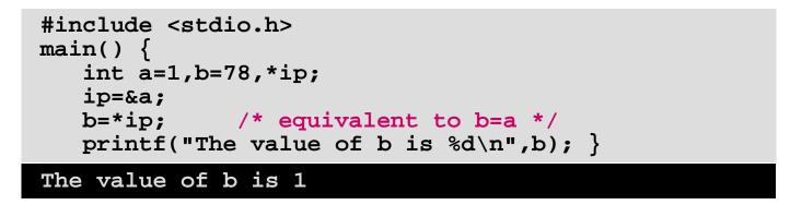
• Note that **b** ends up with the value of **a** but it is done **indirectly**; by using a pointer to **a**.
