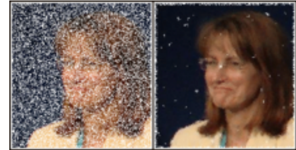
Use of a median filter to improve an image severely corrupted by defective pixels
