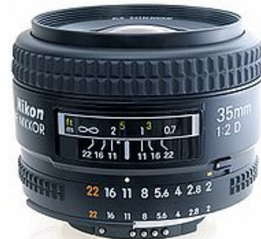
A 35 mm lens set to f/11 , as indicated by the white dot above the f-stop scale on the aperture ring. This lens has an aperture range of f/2.0 to f/22
