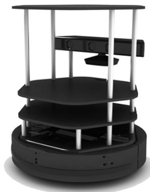
The information from the world is captured by the robot's sensors and we are particularly interested in using visual information from a Kinect camera.
