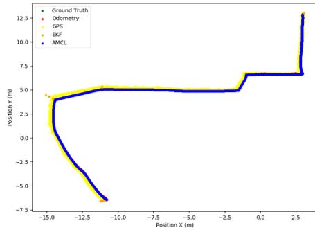
Figure 3: Comparison between the data from sensors/algorithms and ground truth values throughout the path navigated by the AGV.
