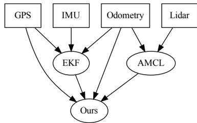
Figure 2: We propose to fuse localization information from two sensors (noisy odometry and GPS) and two prediction methods (AMCL and EKF). Rectangles represent sensors and ovals represent prediction methods. 'Ours' represents the regression approaches evaluated in this work.
