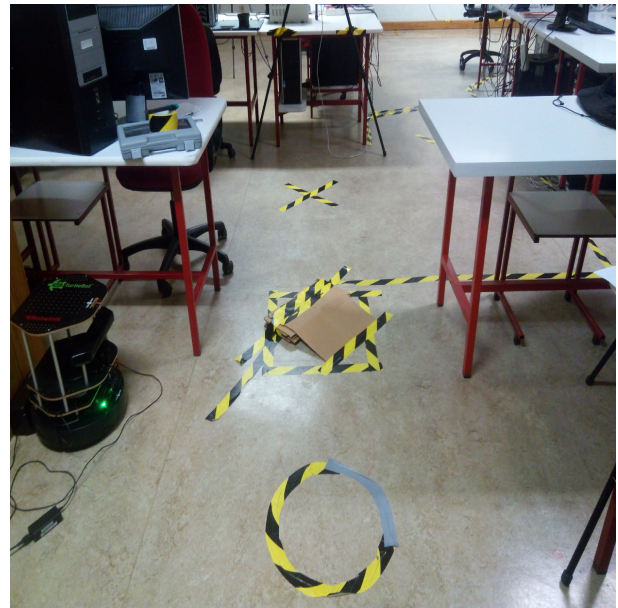
Fig. 2. The turtlebot on its charging dock and the obstacle course. The ramp is low enough so it won't activate the wheel drop sensors that cause the turtlebot to freeze, but high enough to cause slips that confuse the odometry. Also, the entire setup is marked and affixed with duct-tape.
