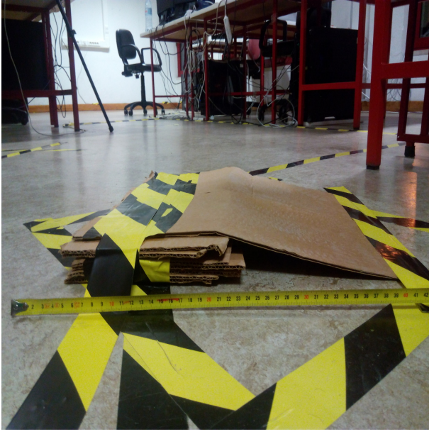
Fig. 3. The obstacle used, made of cardboard with duct-tape binding it all together.
