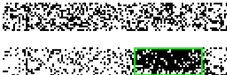
Figure 5.2: Iriscodes matching result illustration. The delimited region correspond to an high concordance area.
