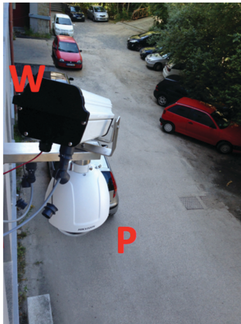
Figure 2.3: Example of a synchronised pair of wide-view (W) and PTZ (P) cameras, from a QUIS-CAMPI laboratorial prototype mounted in the SOCIA: Soft Computing and Image Analysis lab. outdoor wall.
